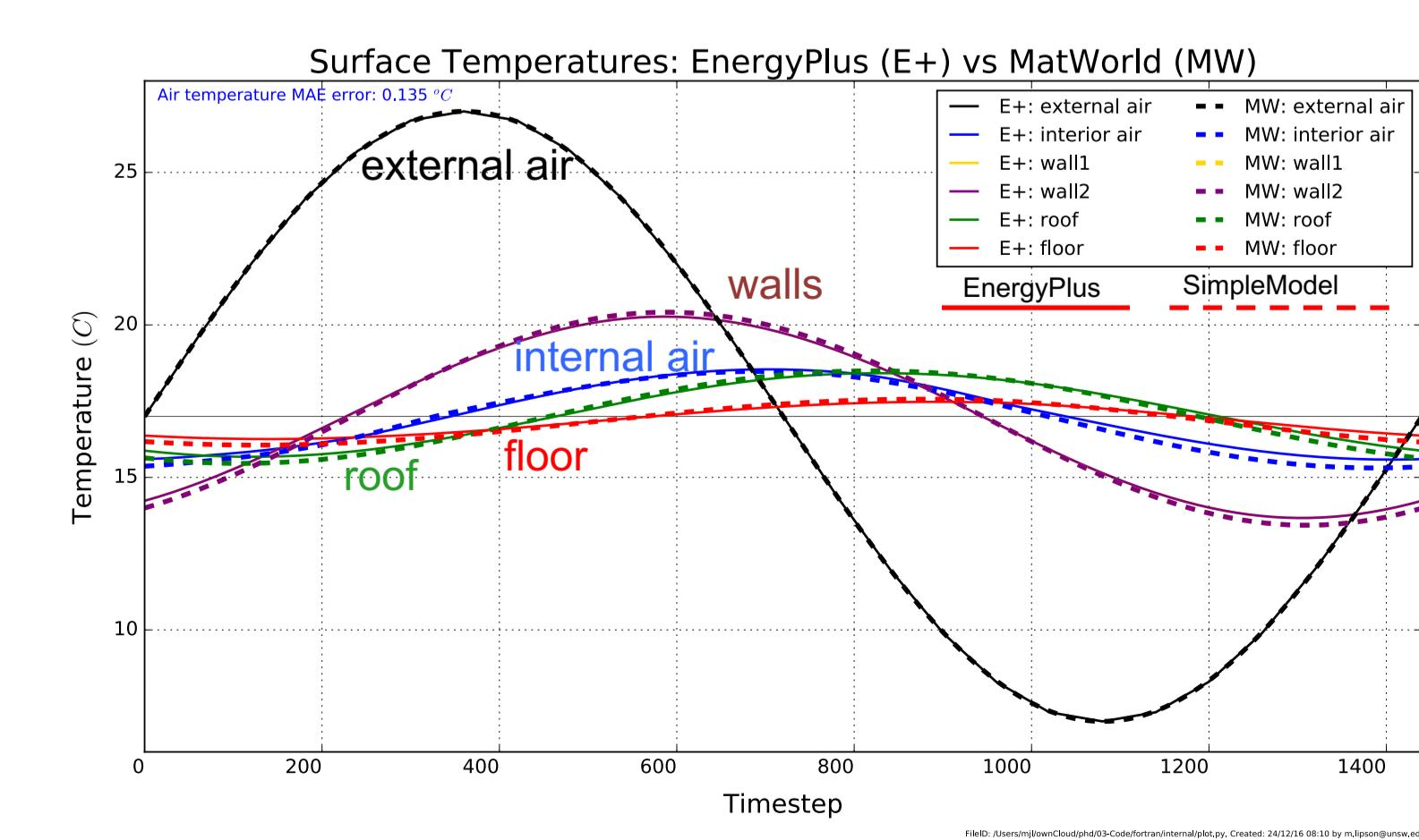
Preliminary Conclusion: Work still underway – so far simple internal model compares well with stripped down EnergyPlus 8.6 model.
